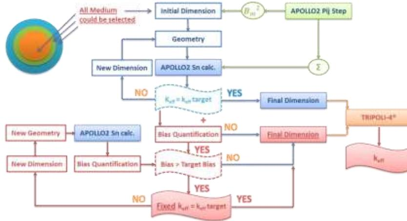
**Figure 3.** Criticality calculation scheme of the standard route
