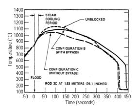
Figure 10: FLECHT-SEASET 21 rods. Centre rod temperature for unblocked and coplanar blockage configurations.
