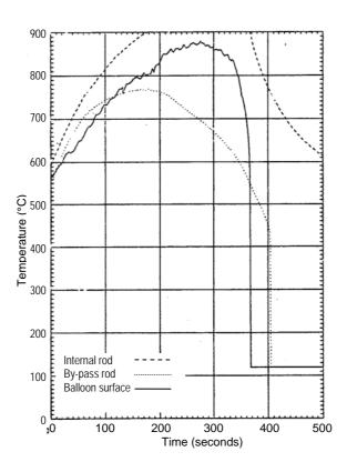
Figure 6: THETIS Run T2R043 80% blockage, 2 cm/s reflood rate
