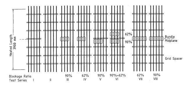
Figure 2: FEBA 5x5 bundle geometries of test series I through VIII
