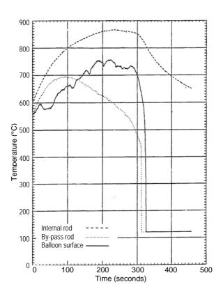
Figure 4: THETIS Run T1R082 3 cm/s reflood rate
