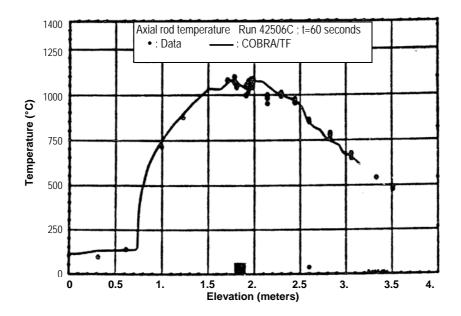
Figure 14: Comparison of COBRA-TF calculated axial rod temperature versus elevation with FLECHT-SEASET 21-rod data, Run 42506C, t=60 s.
