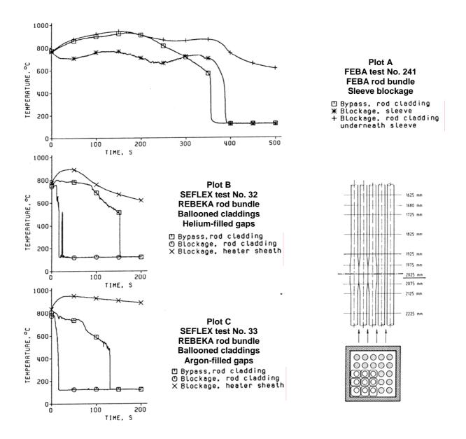
Figure 3: Temperatures measured at the midplane of a 90% blockage and in the blockage bypass of FEBA and SEFLEX rod bundles.
