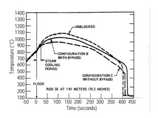
Figure 11: FLECHT-SEASET 21 rods. Peripheral rod temperature for unblocked and coplanar blockage configurations.
