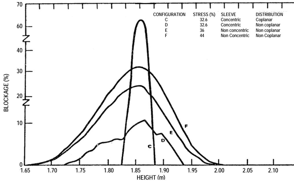
Figure 9: Bundle-wide blockage and axial distributions for FLECHT-SEASET configurations C, D, E and F.
