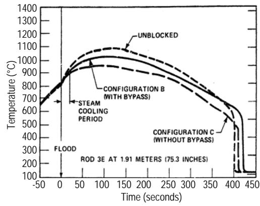
Figure 11: FLECHT-SEASET 21 rods. Peripheral rod temperature for unblocked and coplanar blockage configurations.
