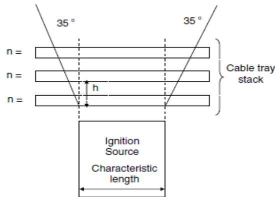
Figure 5: Model for fire propagation in a cable tray stack
