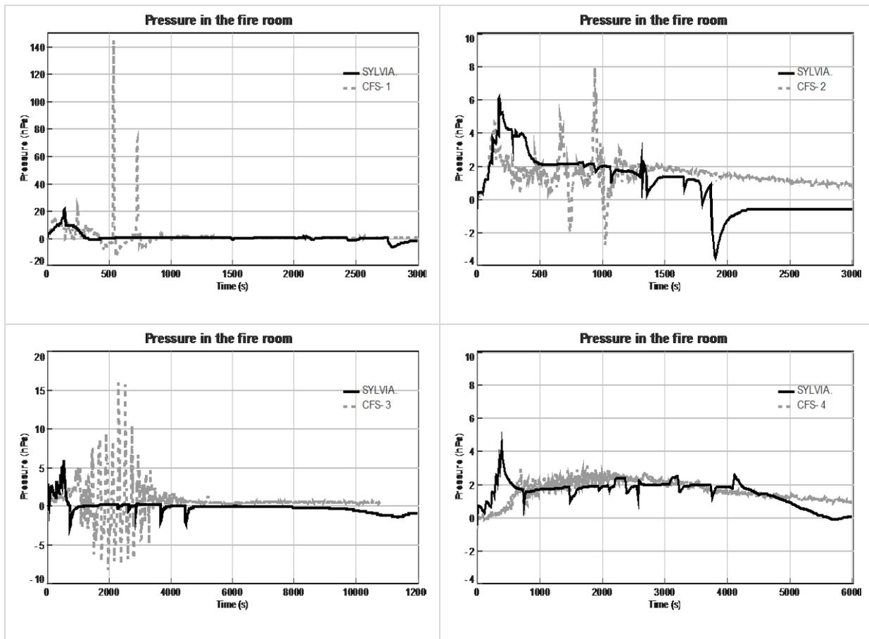
Figure 8: Pressure predictions in the fire room for the CFS tests
