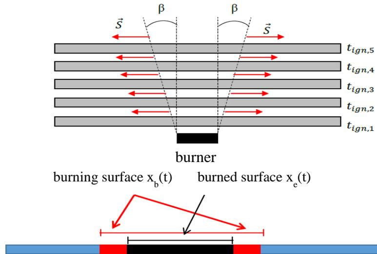
Figure 4: Scheme of the modeling of the burning surface of cables
