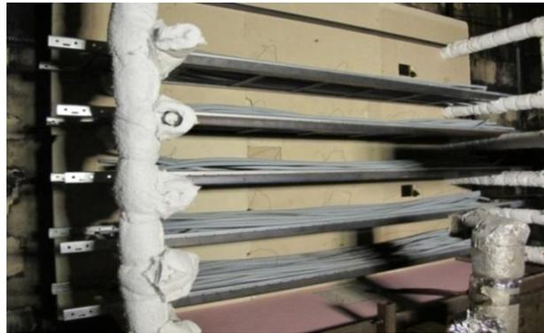
Figure 3: Cable trays fire source
