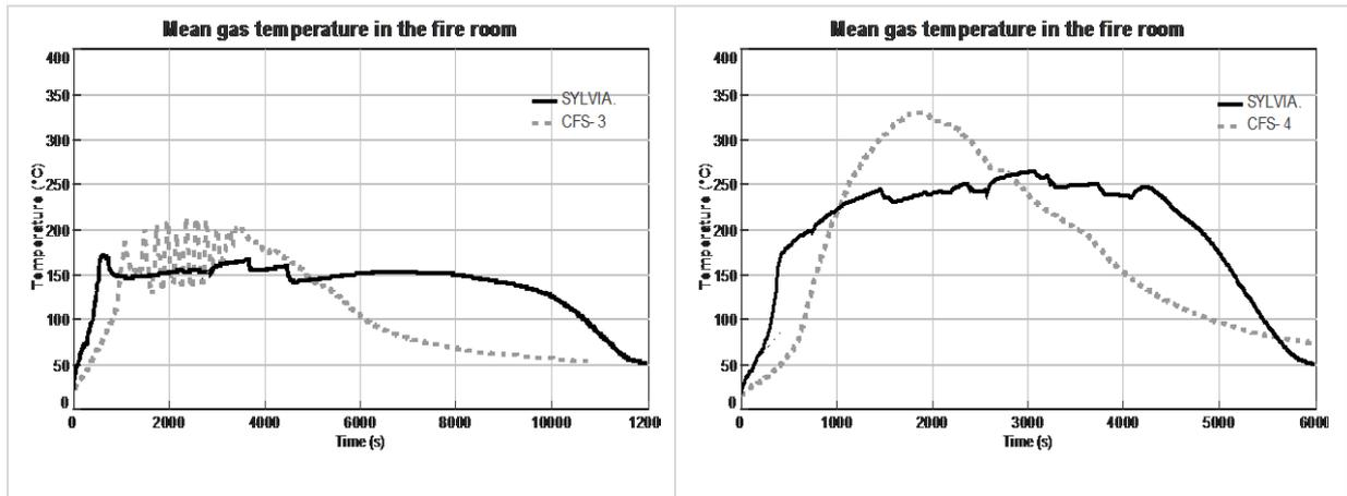
Figure 9: Mean gas temperature predictions in the fire room for the CFS tests
