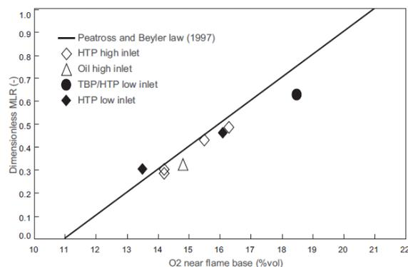
Figure 6: Development of the steady-state fuel mass loss rate with oxygen concentration near the flame base [25]
