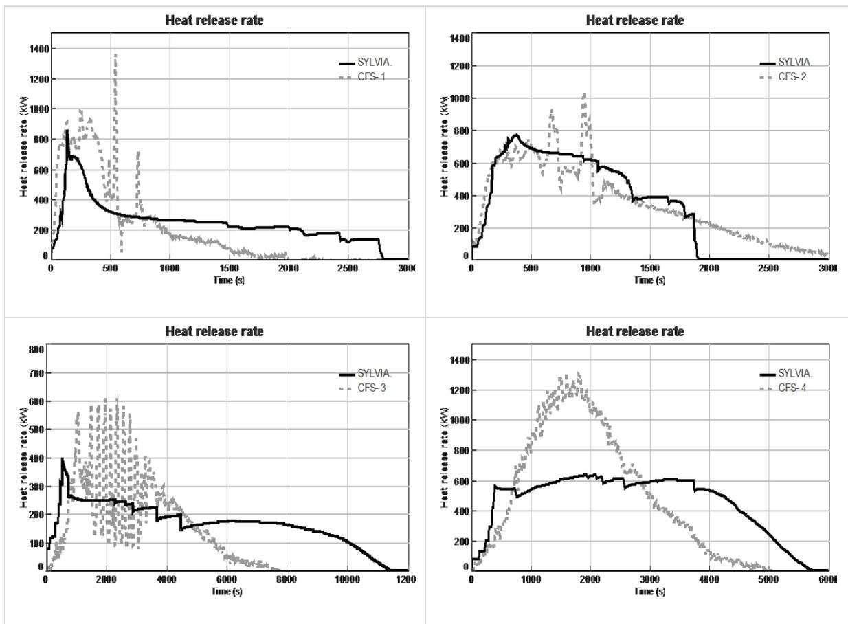
Figure 7: HRR predictions for the CFS tests
