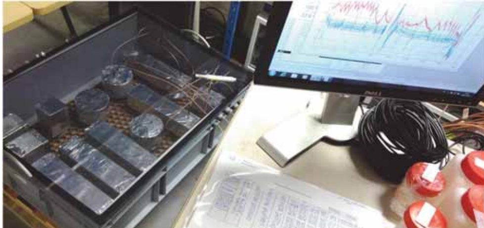
Figure 1: Experimental setup linked to the continuous measurement of RH and T sensors
