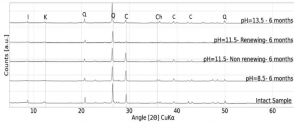
Fig. 7. X-ray diffraction profiles of four Opalinus Clay samples derivate from sample 6 from the lower sandy facies of Mont Terri site immersed in four alkaline solutions for 6 months- I: Illite, K: Kaolinite, Ch: Chlorite, Q: Quartz, C: Calcite.
