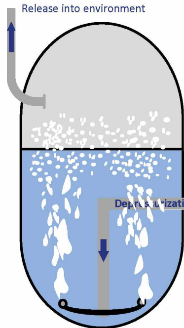
Filtered containment venting system (FCVS)
