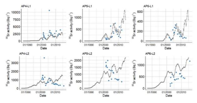
Figure 11. Activity of ion-exchangeable  $^{90}$ Sr measured (circles) and simulated (line) from 1987 to 2015 with the flow-and-transport model in the piezometers located along the cross-sections A-B (R=50).
