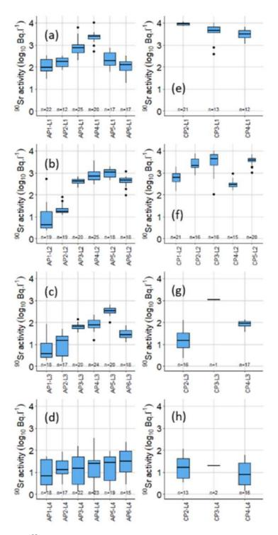
Figure 7. Box-plots of the <sup>90</sup>Sr activities measured in groundwater sampled from 2000 to 2015 in layers L1 to L4 of piezometers (a-d) AP1 to AP6 and (e-h) CP1 to CP5. These plots show the spatial distribution of the <sup>90</sup>Sr activity in the aquifer underlying the trench T22.
