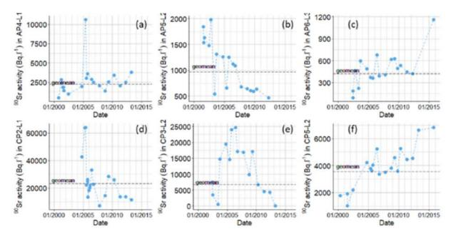
Figure 8. Activity in <sup>90</sup>Sr measured in groundwater sampled from 2000 to 2015 in the <sup>90</sup>Sr plume downstream from the trench T22 in piezometers AP4-L1 (a), AP5-L2 (b) and AP6-L2 (c) and CP2-L1 (d), CP3-L2 (e) and CP5-L2 (f).
