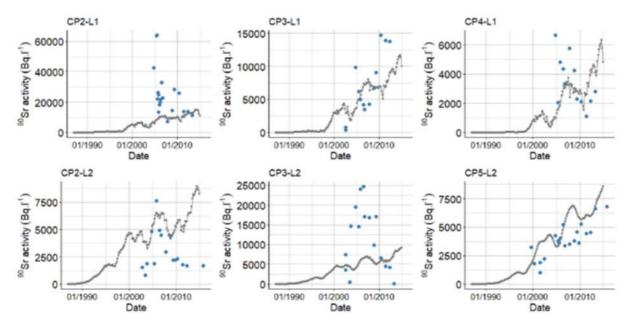
Figure 12. Activity of ion-exchangeable  $^{90}$ Sr measured (circles) and simulated (line) from 1987 to 2015 with the flow-and-transport model in the piezometers located along the cross-sections C-D (R=13).
