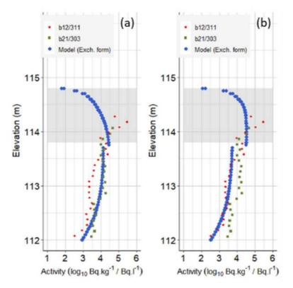
Figure 9. Activity of total <sup>90</sup>Sr and in 2000 measured in samples and of ion-exchangeable <sup>90</sup>Sr simulated with the flow-and-transport model in boreholes b21/303 and b12/311 with (a) R=10; and R=25 (b).
