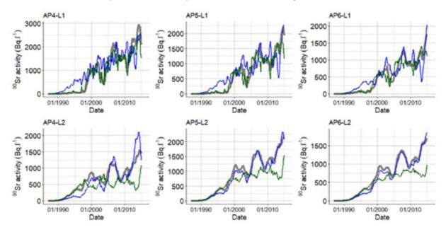
Figure 13. Activity of ion-exchangeable <sup>90</sup>Sr simulated from 1987 to 2015 with the flow-and-transport model in the piezometers located along the cross-sections A-B by considering a temporal variability of both the recharge rate and the groundwater level (grey line); the recharge rate only (green line); the groundwater level only (blue line).
