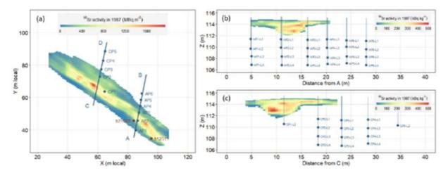
Figure 4. Views of the 3-D model of <sup>90</sup>Sr inventory in 1987 (computed from the mean <sup>137</sup>Cs inventory estimated by Nguyen, 2017) and location of the wells monitored for groundwater activity survey: horizontal view with cumulative <sup>90</sup>Sr activity in depth (a); and views of the A-B (b) and C-D (c) cross-sections.
