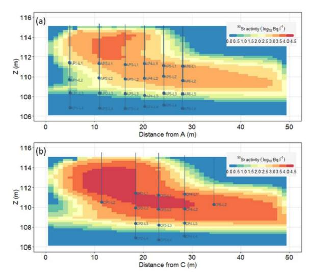
Figure 10. Activity of ion-exchangeable  $^{90}$ Sr simulated in 2015 with the flow-and-transport model along the cross-sections (a) A-B (R=50); and (b) C-D (R=13).
