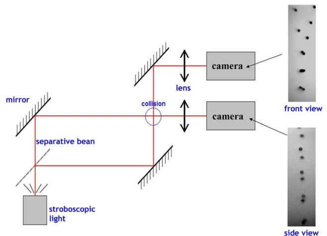
FIG. 3. (Color online) System for recording periodic droplet collisions.
