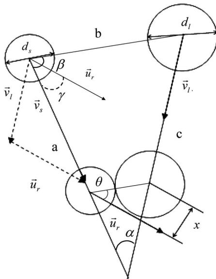
FIG. 1. Sketch of a small droplet (left) and large one (right) before collision and when at contact.  $\alpha$  is the collision angle, (a) and (c) are the distances between the droplet centers before collision and the center of collision, and b is the distance between the droplet centers before collision.
