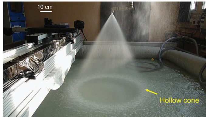
FIG. 6: Annular cross section of the hollow cone spray.
