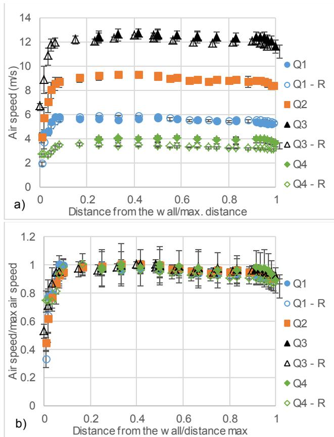
Figure 13. Air speed profiles at different flow rates and their reproduction (a) and nondimensionalized profiles (b)
