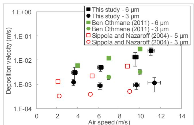
Figure 15. Deposition velocity comparison between this study, [11] and [12] for 2 particle sizes on duct floor
