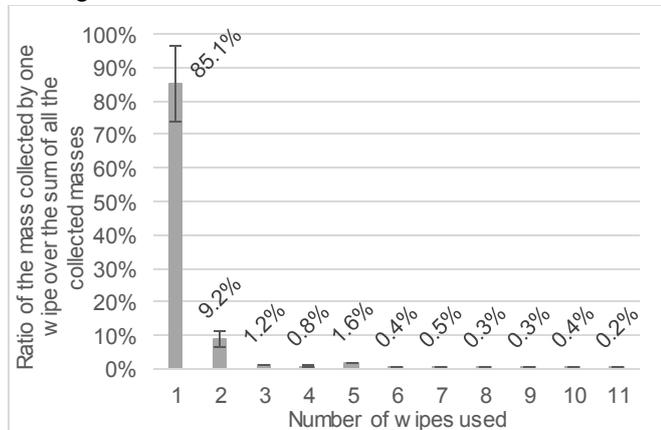
Figure 5. Aerosol collection with each wiping on a galvanized steel surface with deposition around 8 ng/cm<sup>2</sup>
