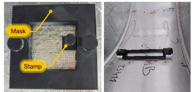
Figure 3. Example of a mask and its stamp (left) and a curved mask fixed on a curved duct (right)
