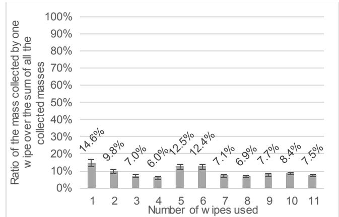
Figure 6. Aerosol collection with each wiping on a galvanized steel surface with deposition around 0.5 ng/cm<sup>2</sup>
