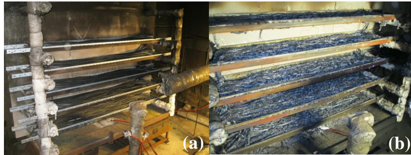
Fig. 10: Cable trays for the CT4 test. (a) before fire. (b) after fire.
