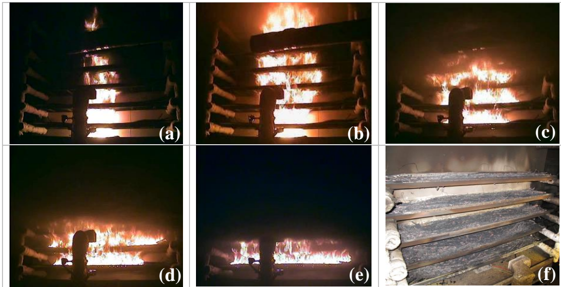
Fig. 9: Cable trays during and after the CT2 test. (a) to (e) during fire. (a) t = 30 s. (b) t = 1 min. (c) t = 2 min. (d) t = 3 min. (e) t = 4 min. (f) after fire.
