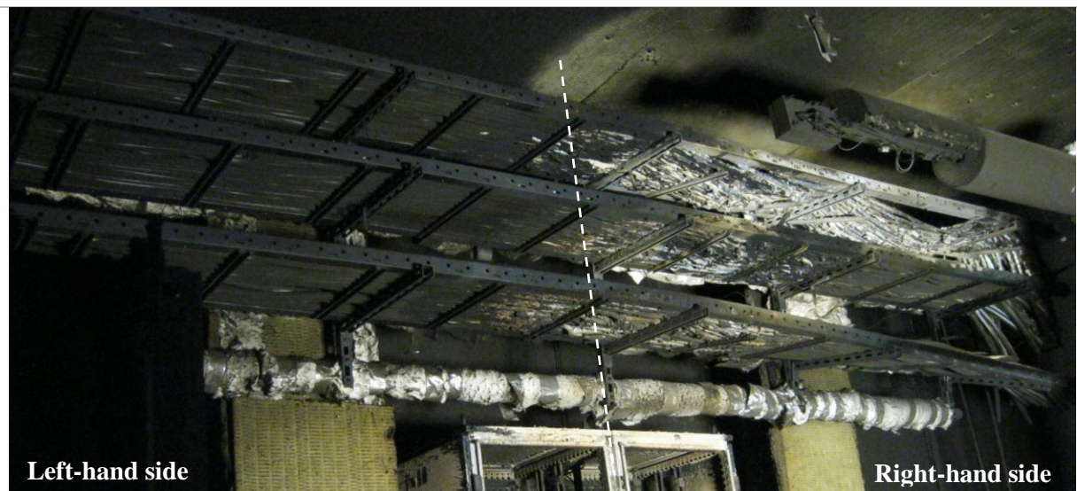
Fig. 16: Global view of the three overhead cable trays after CFS-6 test.
