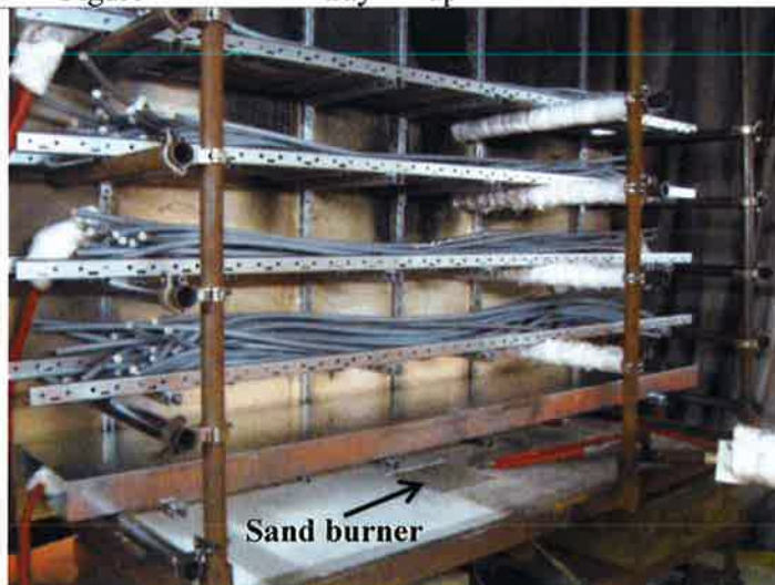
Figure 2: The cable tray set up for the CORE-2 test.
