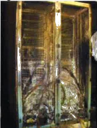
Figure 10: Cable trays after CFS-5.
