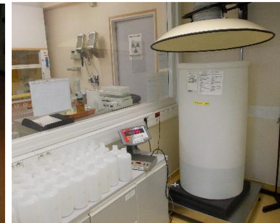
Mixture of water and radioactive solution in an 80L tank
