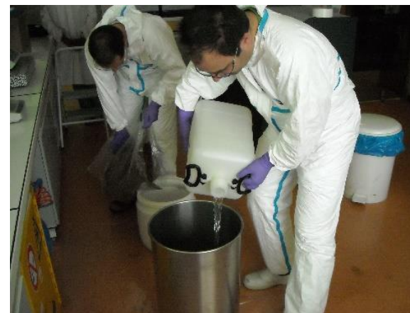
Impregnation of a radioactive solution on commercial tea
