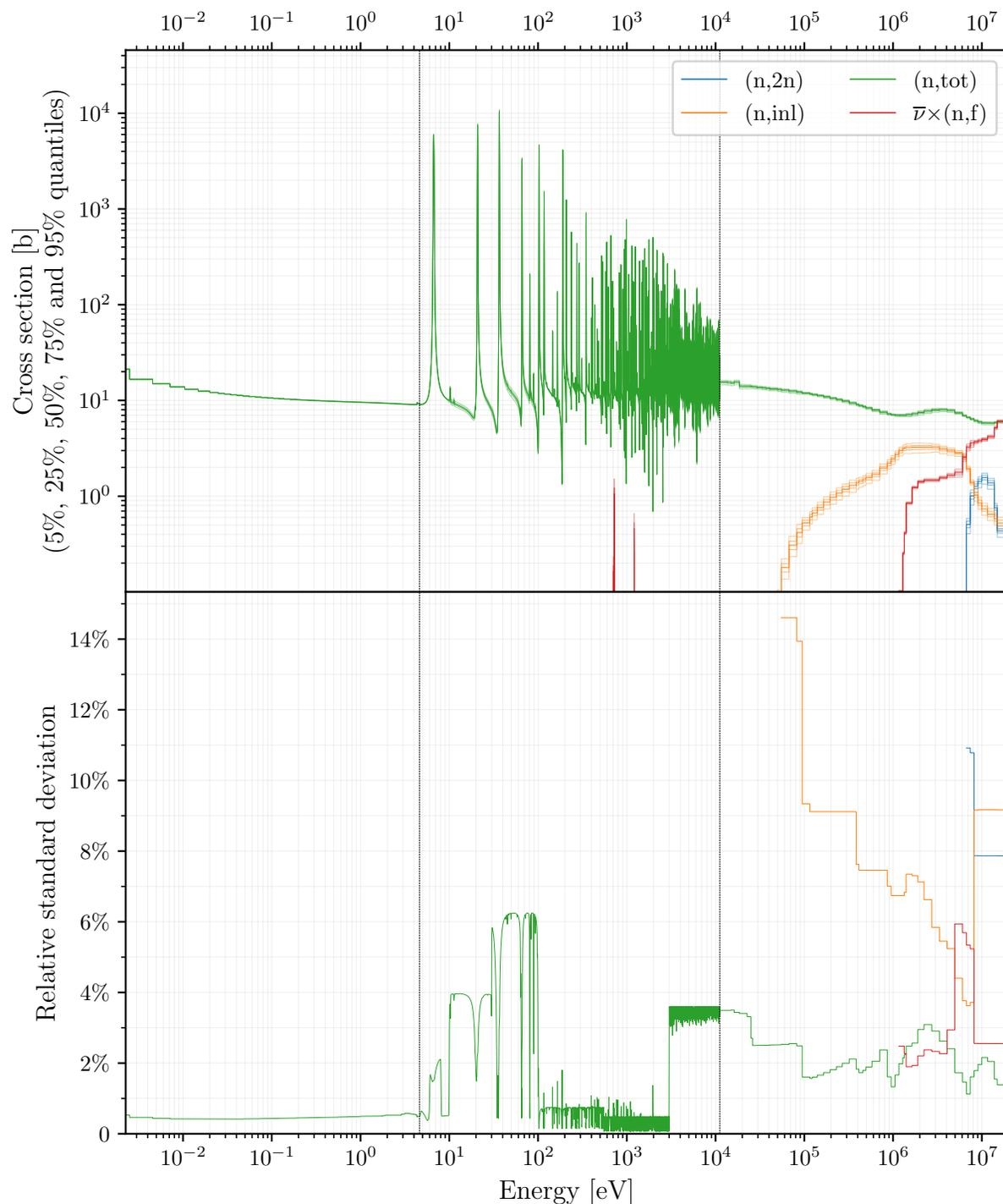
**FIGURE 3 – Uranium 238 cross sections statistics of 300 samples within JEFF-3.3. The temperature is 550 K (276.85°C). The continuous plotted data are those contained in the DRAGLIB files, as used by DRAGON5, allowing it to reach excellent accuracies [27] (computing on-the-fly mathematical probability tables for self-shielding subgroup methods). Plotting instructions are openly available [28], along with the released data itself [26].**
