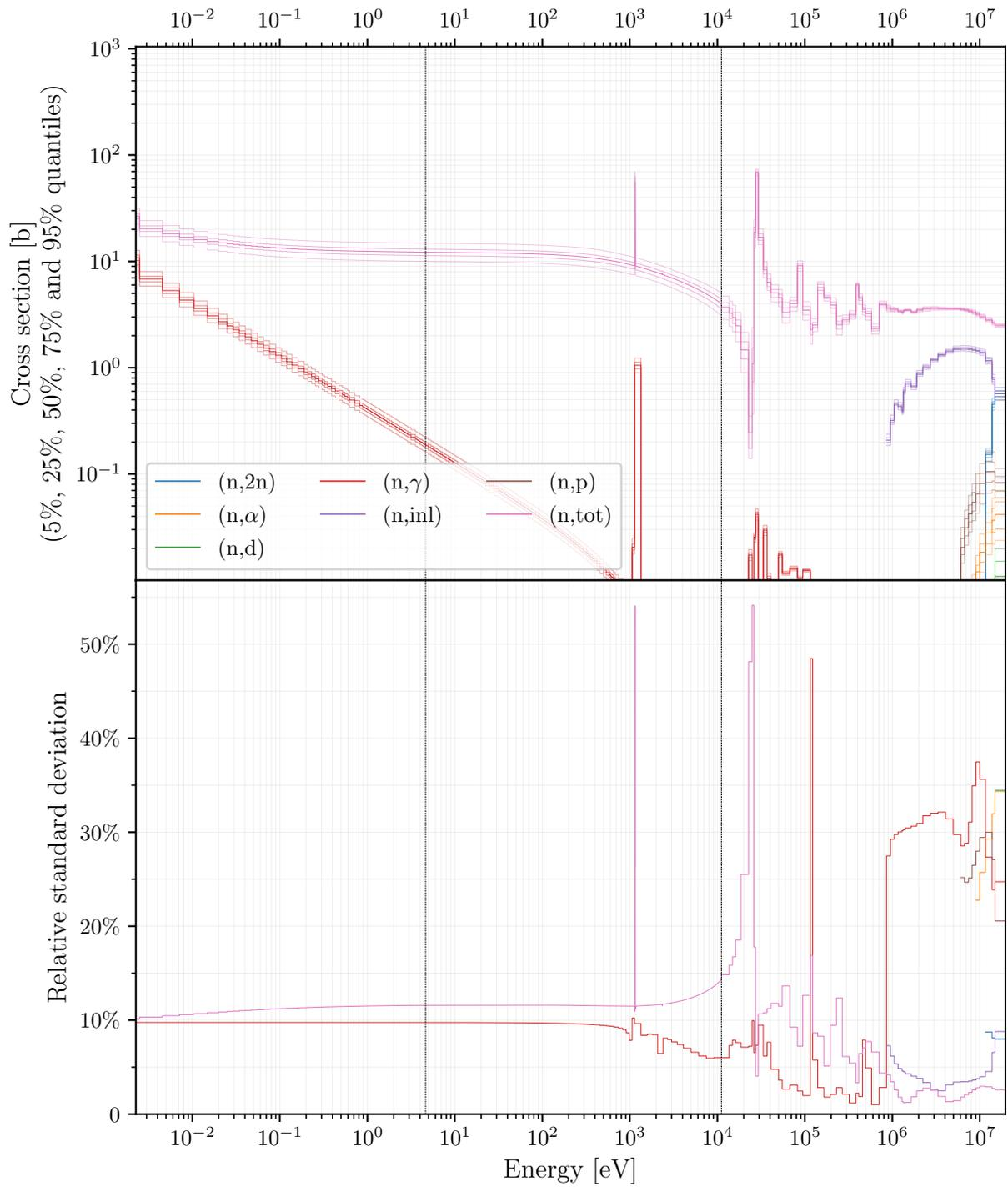
**FIGURE 4 – Iron 56 cross sections statistics from 300 TENDL-2019 files, presampled upstream of its nuclear physics models. The temperature is 550 K (276.85°C). Plotting instructions are openly available [28], along with the released data itself [26].**
