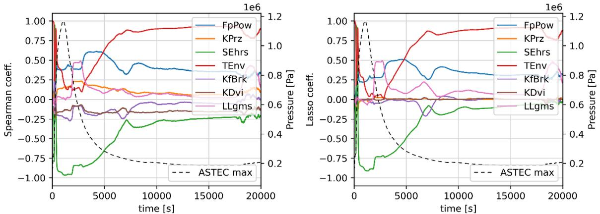
Fig. 4: Spearman (left) and Lasso (right) coefficients for DW pressure.
