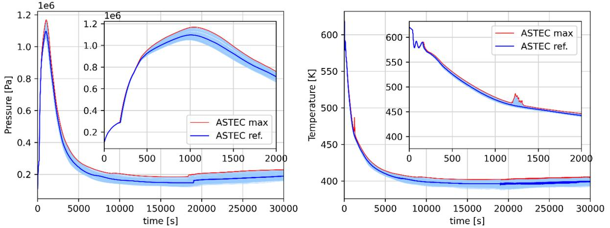
Fig. 3: Uncertainty band of the DW pressure (left) and of maximum cladding temperature (right).
