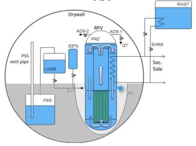
Fig. 1: Scheme of the main components and passive safety systems for a generic IRIS reactor [4].
