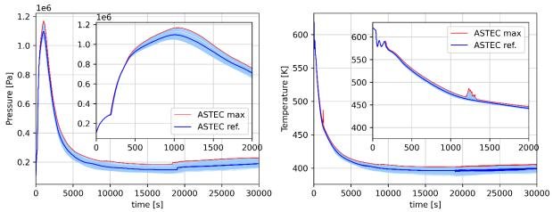
Fig. 3: Uncertainty band of the DW pressure (left) and of maximun cladding temperature (right).
