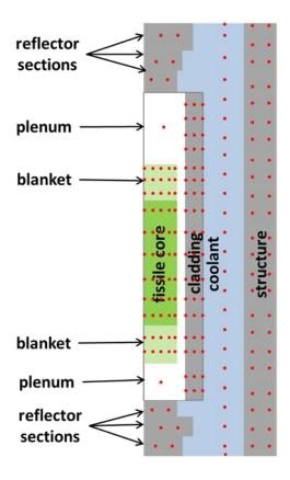
Figure 3 Axial Node Structure used in SAS-SFR code
