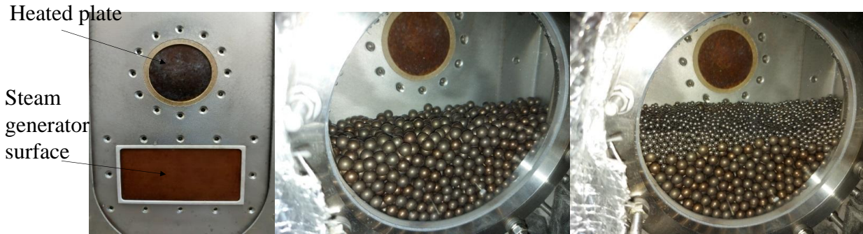
Figure 4. Inside View of the Ball Bed Progressive Filling – Empty (Left), Large 8 mm Balls in front of SG (Center) and 4 mm Balls in the Rest of the Bed (right: picture is taken before the complete filling up to the heated plate).
