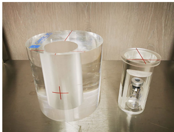
Fig. 1 Neck phantom for thyroid cross-calibration factor determination for the planar, SPECT/CT and SPECT acquisitions
