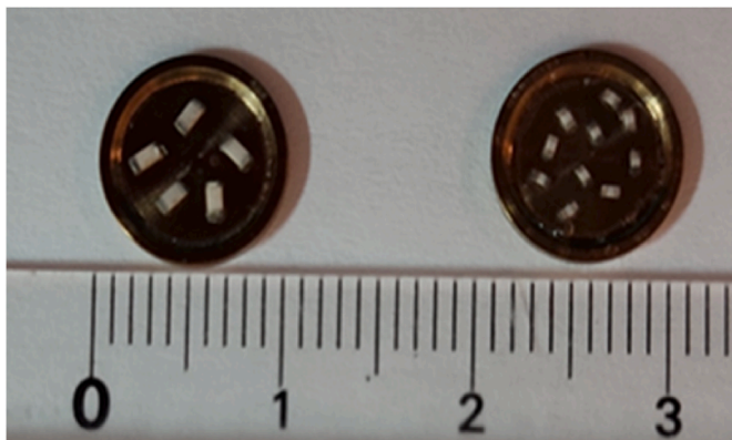
Fig. 1. A cup of five electronic components from a portable radio investigated in this study (on the left) and a cup of ten resistors (type 0402) from a mobile phone (on the right).
