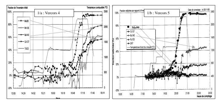
Figure 1: Vercors 4 and 5 release kinetics (% of the initial inventory after irradiation) for Cs, Mo, and Ba.
