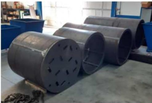
Fig. 7. Confinement tube composed of four sections.
