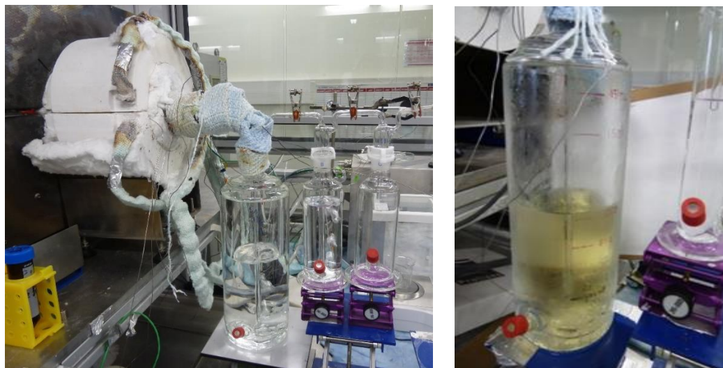
Fig. 2 START2 test facility (left) and RuO 4 dissolved in alkaline solution with the higher liquid trap – steam conditions (right)
