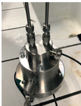
a) Fig 1 Self-sealing test (a) View of the testing cell. b) First results. Evolution of fissure closure as a function of time.
