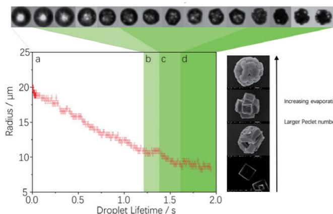
An example of evaporation profile for NaCl solution aerosol with an initial concentration of  $50\text{g}\cdot\text{L}^{-1}$  in a dry nitrogen environment at 296 K. The different stages of the drying process are marked by shading – initially a homogeneous droplet, followed by an inhomogeneous droplet stage, then a stage of a semi-crystalline particle and finally a dry crystalline particle. Example dry NaCl morphologies are shown on the right.
