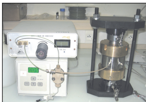
Figure 1 : cellule de percolation
