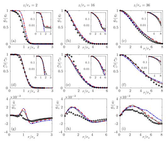
FIGURE 4. Radial evolution of the mean streamwise velocity (a,b,c), the mean concentration (d,e,f) and the mean radial velocity (g,h,i). The distance to the source of the jet is fixed to  $z/r_s = 2$  (a,d,g),  $z/r_s = 16$  (b,e,h) and  $z/r_s = 36$  (c,f,i). Same symbols and lines as in figure 3.
