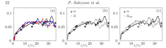
FIGURE 9. (a) Axial evolution of the entrainment coefficient  $\alpha$  for simulations (black dotted lines: J1a, red dashed lines: J2, blue dot-dashed lines: J3) and experiment (symbols). In (b) and (c),  $\overline{\alpha}$  defined by (5.4) and  $\overline{\alpha}_{ap}$  defined by (5.5) are also plotted against  $z/r_s$  for simulation J1a and experiment.
