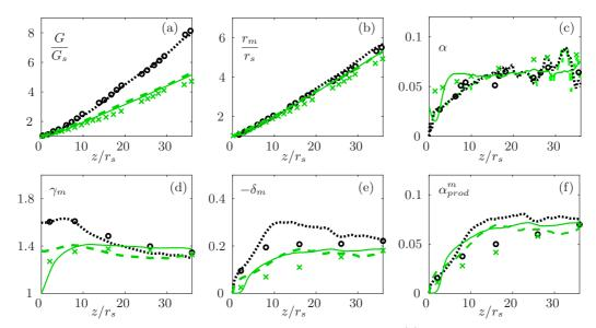
FIGURE 12. Longitudinal profile of the non-dimensional mass flux (a), mean characteristic radius (b), entrainment coefficient estimated by (2.12) (c), mean profile coefficients  $\gamma_m$  (d) and  $-\delta_m$  (e), and  $\alpha_{prod}^m$  (see eq. 5.6) (f), for the low-density jet (J1a, black dotted line and circles) and the iso-density jet (J0, green dashed line and crosses). Also shown: DNS of van Reeuwijk et al. (2016) for an iso-density jet (green solid line).
