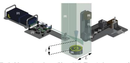
FIGURE 2. Sketch of the experimental set-up (Moutte 2018). The main elements are as follows: camera for PIV (0), 200mm lens (1), pulsed laser (2), camera for PLIF (3), 532nm optical filter (4), light intensifier (5), dichroic mirror (6), optical table (7), containment box (8), jet maker (9).
