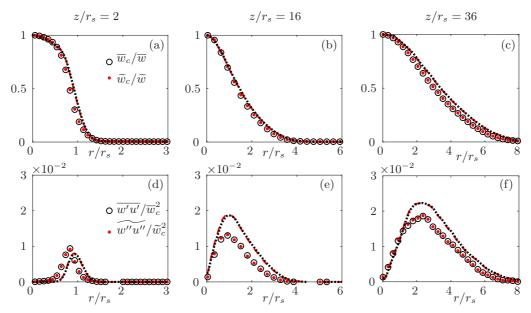
FIGURE 7. Effect of the Reynolds or Favre averaging on the radial evolution of the mean streamwise velocity (a,b,c) and Reynolds stress (d,e,f). The distance to the source of the jet is fixed to  $z/r_s=2$  (a,d),  $z/r_s=16$  (b,e) and  $z/r_s=36$  (c,f). Symbols: experiments. Lines: reference simulation (J1a). Black circles and dotted lines: Reynolds averaging. Red dots and lines: Favre averaging.
