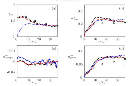
FIGURE 11. Longitudinal profile of the mean profile coefficients  $\gamma_m$  (a),  $-\delta_m$  (b),  $\alpha_{shape}^m$  (c) and  $\alpha_{prod}^m$  (d). Circles: experiments. Black dotted lines: reference simulation J1a. Red dashed lines: J2 (without bottom wall and using top-hat profile for the inlet velocity). Blue dot-dashed lines: J3 (with bottom wall and using top-hat profile for the inlet velocity).
