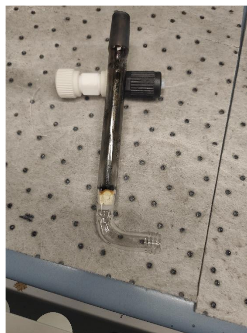
Figure 9: Sintered column containing UiO-66-NH 2 after MOF-H test.
