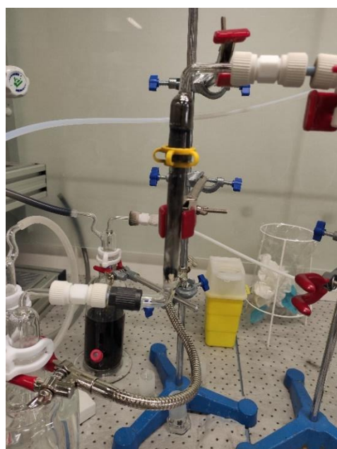
Figure 9: Sintered column containing UiO-66-NH 2 after MOF-H test.
