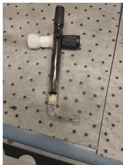
Figure 9: Sintered column containing UiO-66-NH 2 after MOF-H test.
