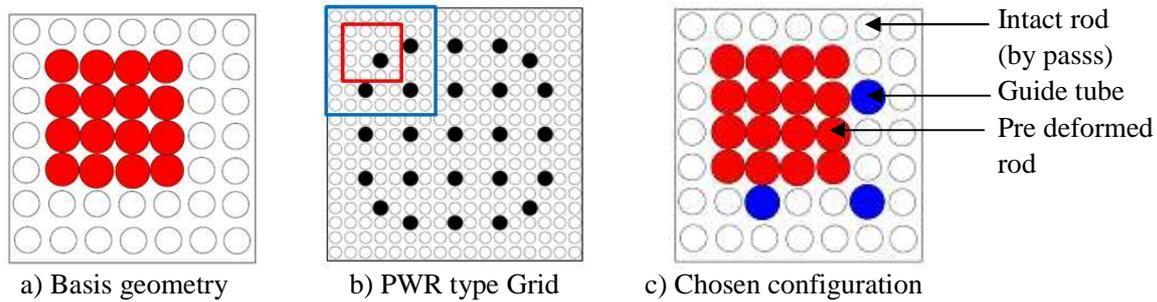
**Figure 3. Typical bundle fuel rods for COAL experiments**
