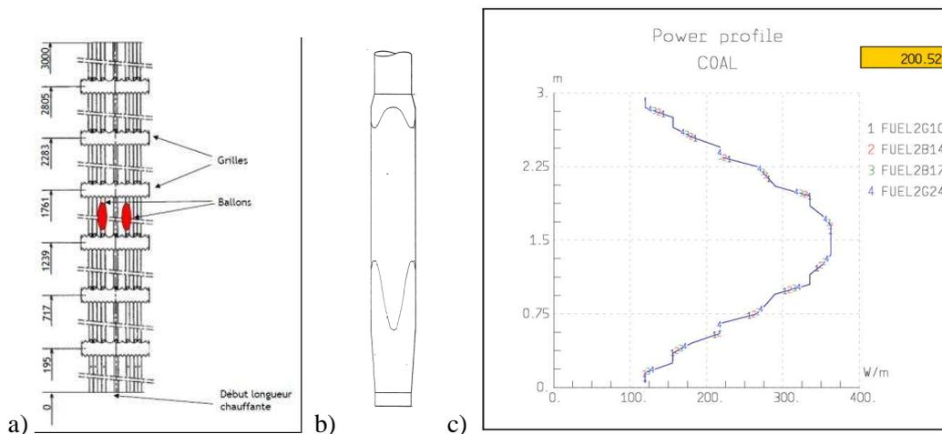
Figure 9. Axial position of the blockage area
