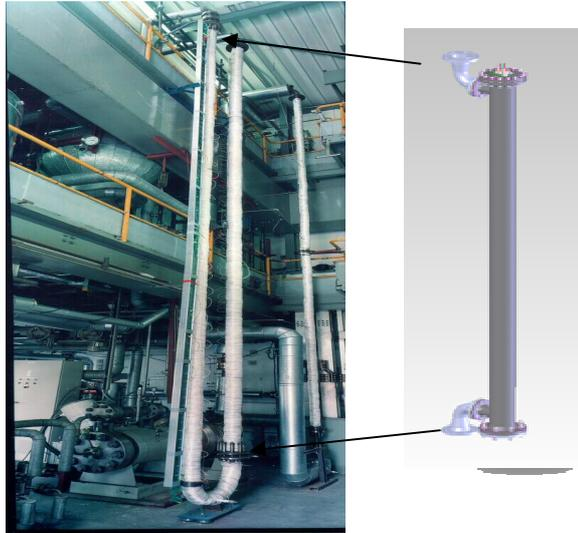
**Figure 7. BENSON facility at Erlangen and COAL Test Section**
