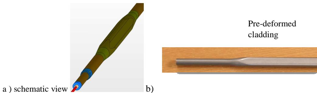
**Figure 4. Electrical deformed fuel rod prototype (SAFRAN)**
