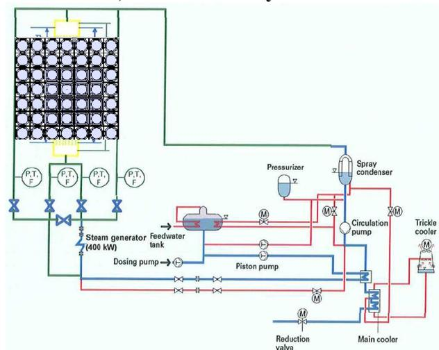
**Figure 6. COAL test bundle and circuit of the BENSON facility**
