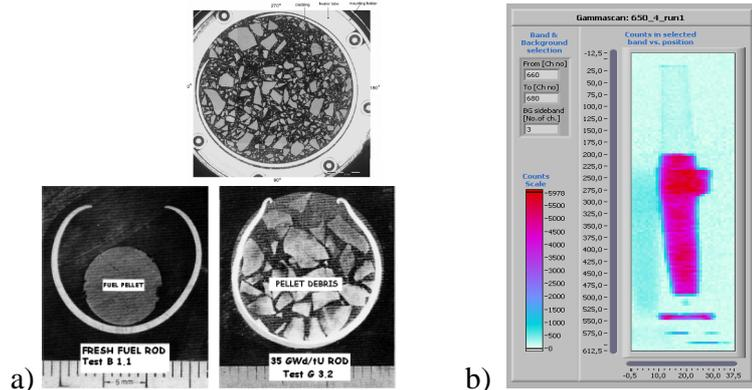
**Figure 2. Fuel relocation in the ballooned area
