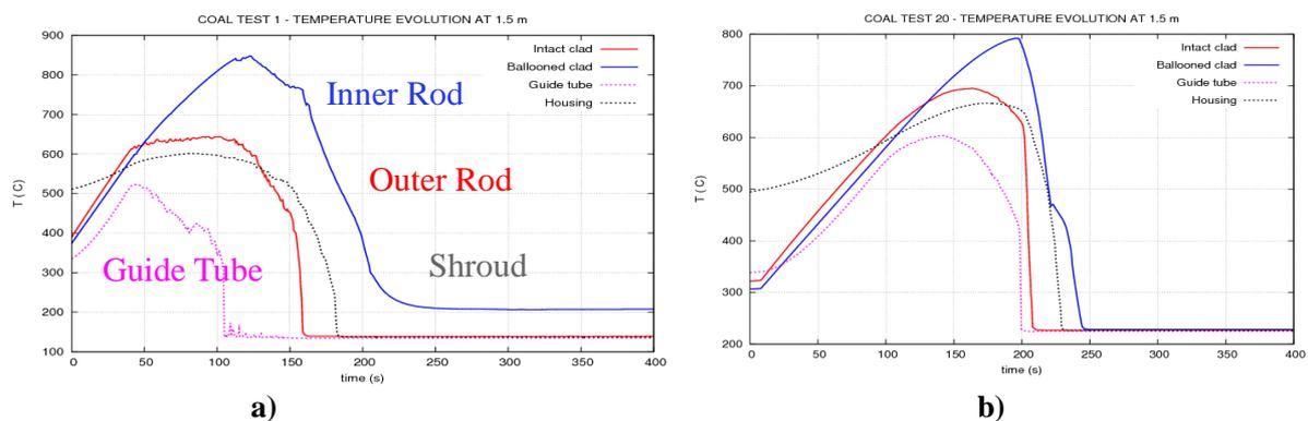
**Figure 14. DRACCAR preliminary Calculations for deformed bundle geometry - Clad temperature evolution at 1.5 m for intact bundle geometry for a) Large break LOCA reflooding (3bar) and b) for Intermediate break LOCA (25 bar).**
