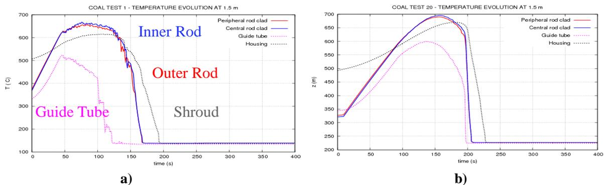
**Figure 13. DRACCAR preliminary Calculations for intact bundle geometry - Clad temperature evolution at 1.5 m for intact bundle geometry for a) Large break LOCA reflooding (3bar) and b) for Intermediate break LOCA (25 bar).**
