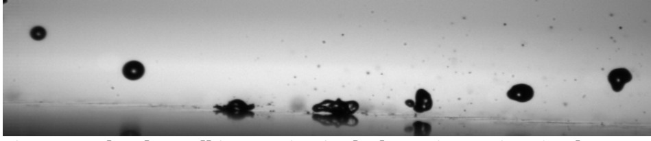
Figure 14: droplet-wall interaction in the bouncing regime (Weber < 40)
