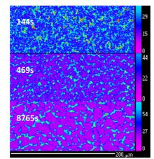
Figure 6- Phase  $\alpha$  (purple) and phase  $\beta$  (light blue) distribution as a function of time exposure at 850°C.
