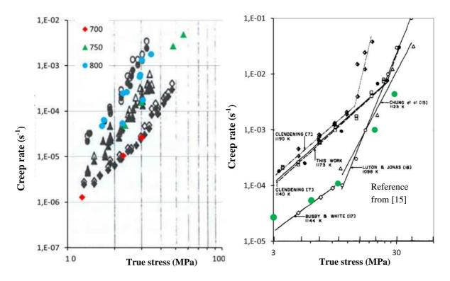
Figure 5- True strain as a function of true stress: a) Tests performed between 700 and 800°C versus Frechinet results ; b)Test performed at 850°C versus Rosinger's data collection
