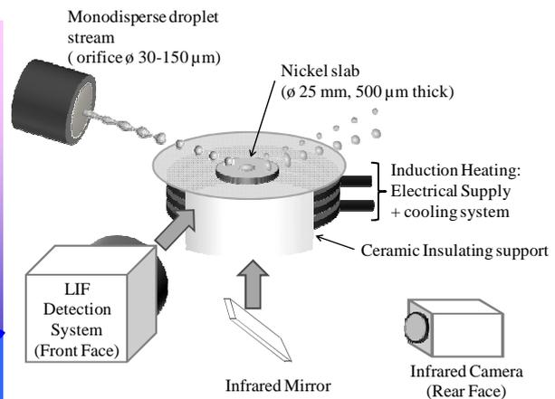
Figure. 13: Temperature measurement
