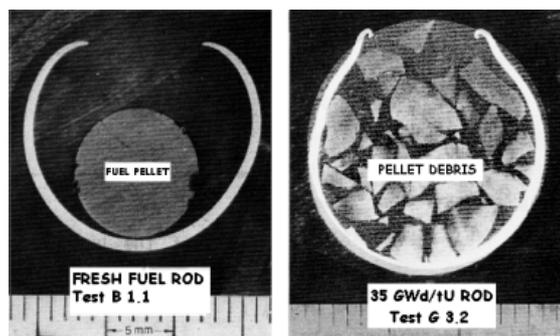
**Figure 2. Fuel relocation in the ballooned area
