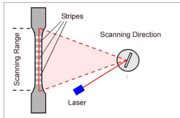
Figure 4: measurement of the deformation
