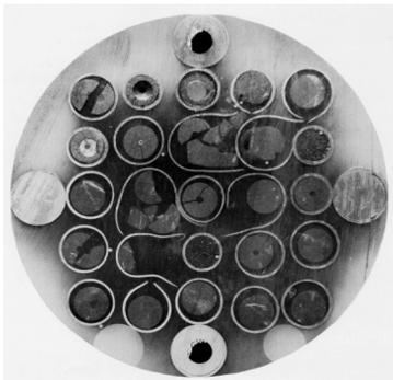
**Figure 1. Bundle of deformed fuel rods
