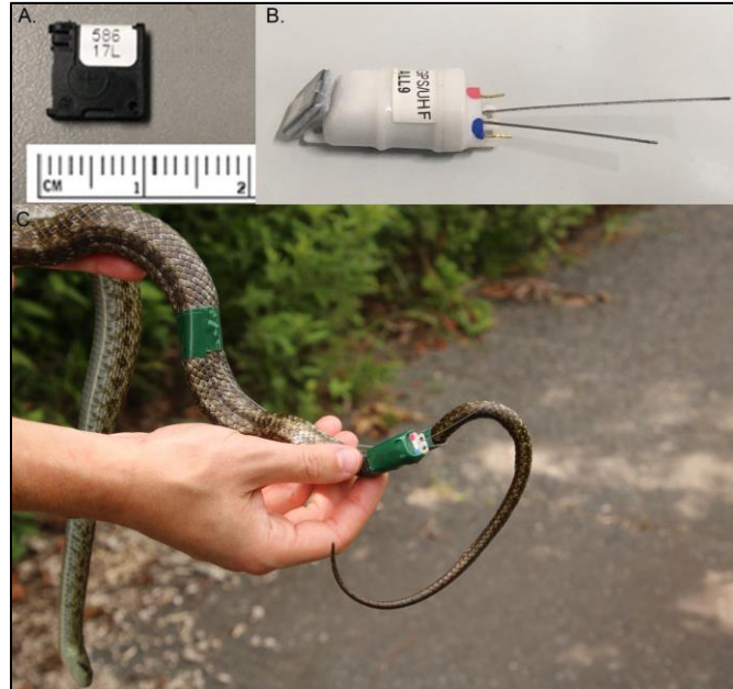
Figure 3. Photo of: A) optically stimulated luminescence (OSL) dosimeter, B) OSL dosimeter attached to GPS/UHF transmitter, and C) VHF transmitter and GPS/ UHF transmitter with OSL dosimeter on the tail of a Fukushima snake (Gerke et al., 2020).
