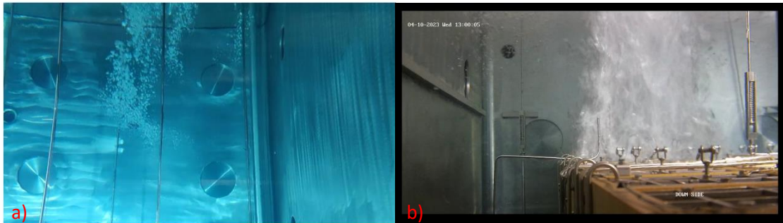
Figure 7: Vapor bubbles produced by gravity-driven flashing of superheated water (a). Vapor bubbles generated by nucleate boiling (b).
