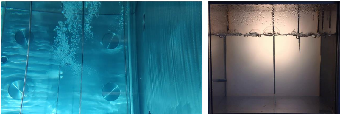
Figure 4: Observation of the gravity-driven pool flashing phenomenon in two test facilities of different scale, operated at IRSN. Left: MIDI test device. Right: Aquarius test device [16], [17].
