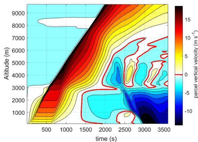
**Figure 5.** Spatial–temporal distribution of the vertical components of atmospheric flows. The thick line in red separates the updraught ( $w_{\text{air}} > 0$ ) flows from the downdraught flows ( $w_{\text{air}} < 0$ ).
