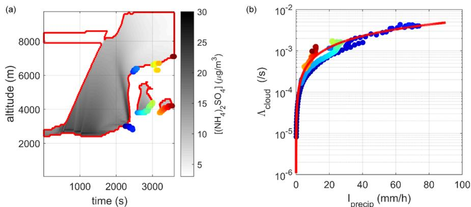
**Figure 8.** (a) Spatial–temporal distribution of the ammonium sulfate concentration in the cloud contour (the solid line shows the cloud contour for a relative humidity greater than 80 %). (b) Correlation between the scavenging coefficient and the precipitation intensity determined at the base of the cloud, adjusted by a power law (solid line).
