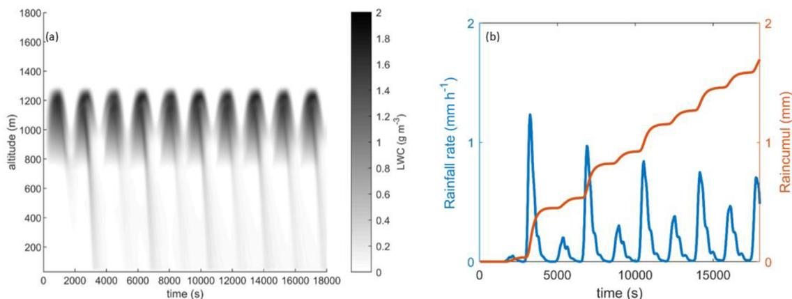
**Figure 12.** (a) Spatial–temporal distribution of the liquid water content calculated by DESCAM (LWC, in greyscale). (b) Temporal evolution of rainfall intensity and cumulative precipitation diagnosed by DESCAM at ground level.
