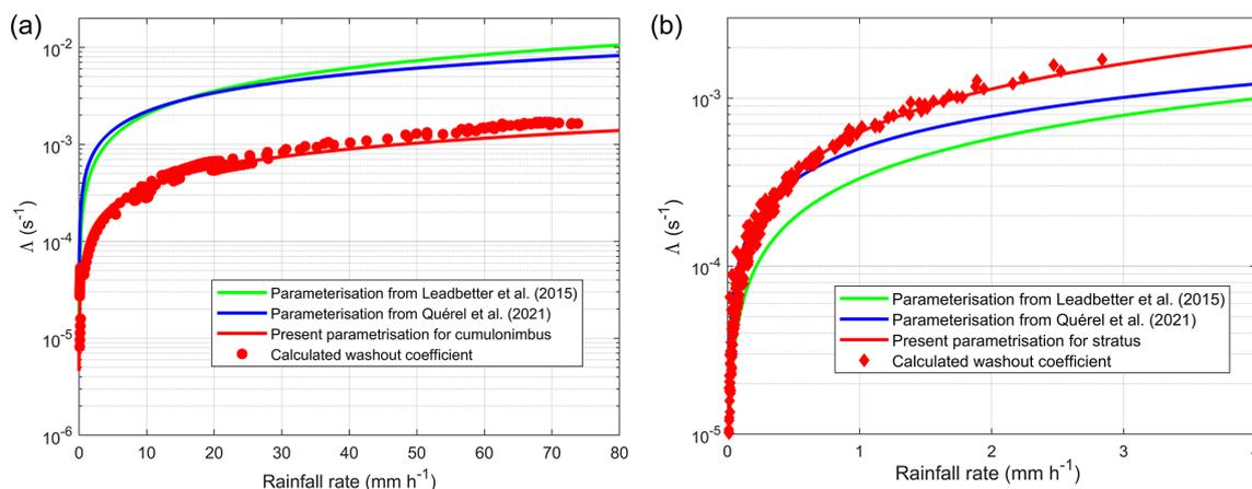
**Figure 18.** Comparison of the parameterisations established for a cumulonimbus (a) and a stratus (b), with the parameterisations established by Leadbetter et al. (2015) and Quérel et al. (2021) following the Fukushima accident.
