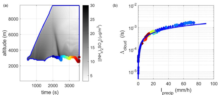
**Figure 10.** (a) Spatial–temporal distribution of the ammonium sulfate concentration in the cloud contour (the solid line shows the cloud contour for a concentration in the number of hydrometeors greater than  $0.003 \text{ particles cm}^{-3}$ ). (b) Correlation between the scavenging coefficient and the precipitation intensity determined at the base of the cloud, adjusted by a power law (solid line).
