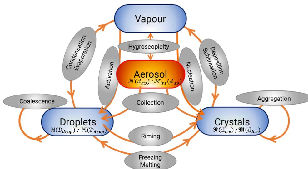
**Figure 2.** Modelling of microphysical processes in DESCAM.
