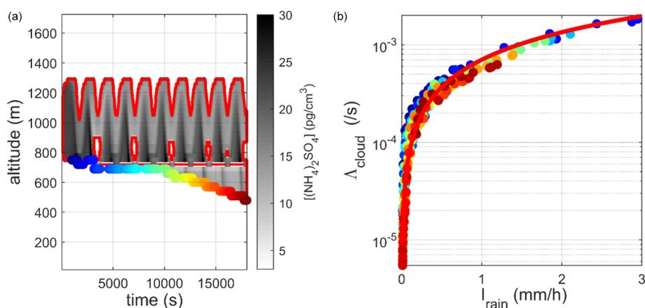
**Figure 15.** (a) Spatial–temporal distribution of the ammonium sulfate concentration in the cloud contour (— cloud contour for a relative humidity above 99 %). (b) Correlation between the scavenging coefficient and the precipitation intensity determined at the base of the cloud, adjusted by a power law (—).
