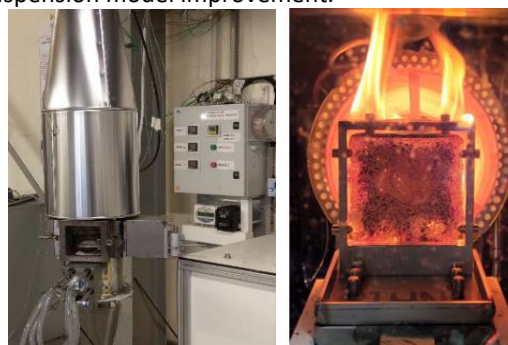
Figure 1. Left: ARTEMIS facility. Right: Thermal degradation of a polycarbonate sample in ARTEMIS.
