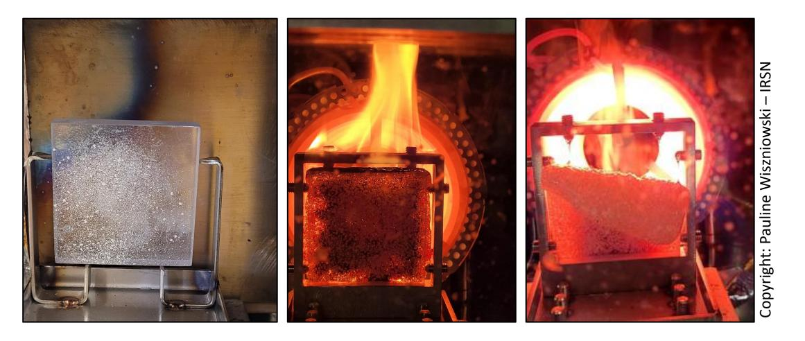
Bubbles appear on the surface of the polymer during the first phase of the fire. Then, the sample ignites. The sample ultimately collapses due to its deformation and loss of mechanical integrity after reaching its glass transition temperature. It is followed by the formation of a carbonaceous residue.
