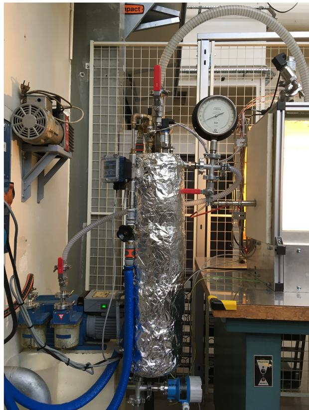
Figure 2.11: Front-view of the condenser equipping the test device, coated by a rock-wool thermal insulation layer.
