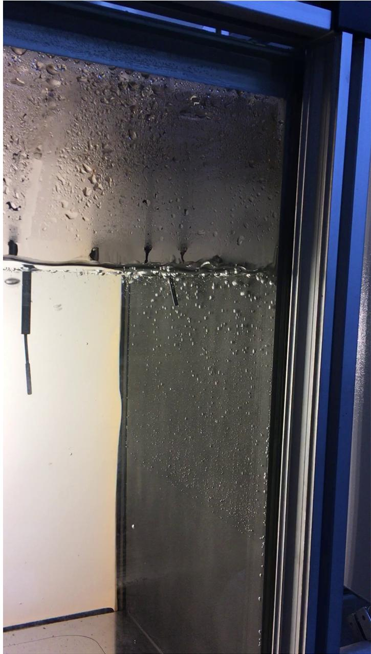
Figure 3.65: A study of the forcing of bubble nucleation onto the unheated rough wall of the vessel. Photo taken during the bubbling stage of the test conducted at a power of 250 W, a pressure of 22 mbar, an initial dissolved  $O_2$  concentration of 9.5 mg/L, an initial pool level of 30 cm and a prior dry out of the unheated rough wall. During the beginning of that stage, bubbles were seen nucleating both within the liquid bulk and onto the pre-dried out wall.
