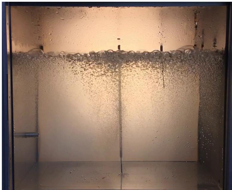
Figure 3.7: After about 1 min, some bubble nucleation appeared as well onto the left-side of the heated wall. At that moment, the flow seemed to re-organize through the form of a central bubbly plume, most likely composed of the merge of the plumes generated right on top of the two sides of the heated surface.
