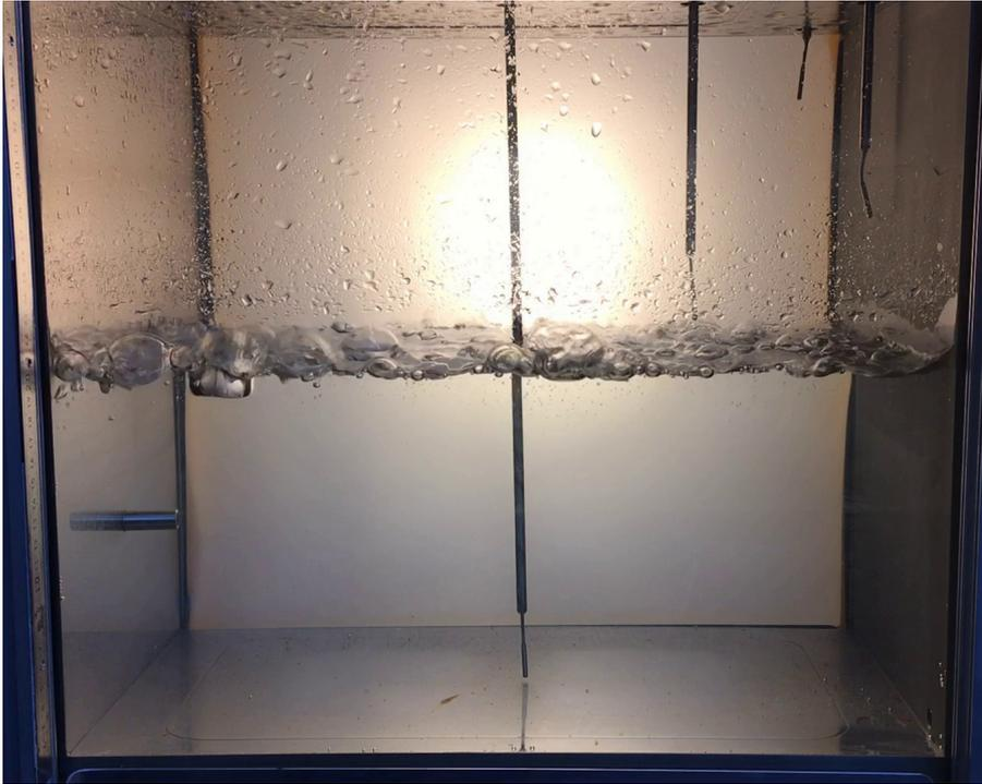
Figure 3.46: A photo taken 3 min after the beginning of the test conducted at a power of 250 W, a pressure of 22 mbar, an initial dissolved  $O_2$  concentration of 6.5 mg/L and an initial pool level of 20 cm, exhibiting some strong flashing underneath the liquid free surface.
