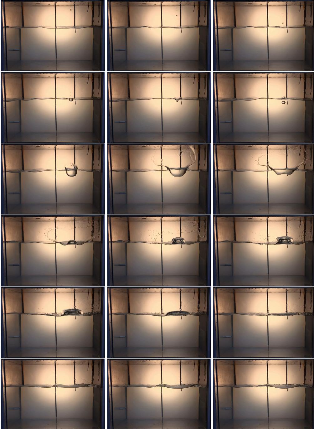
Figure 4.27: A series of photographs taken during the late stage of the reference test, presented in Chapter 3. The pictures are displayed every 4 ms. The series shows the interaction of a falling droplet with the free surface of the superheated liquid. The interaction leads to the violent growth of a bubble.
