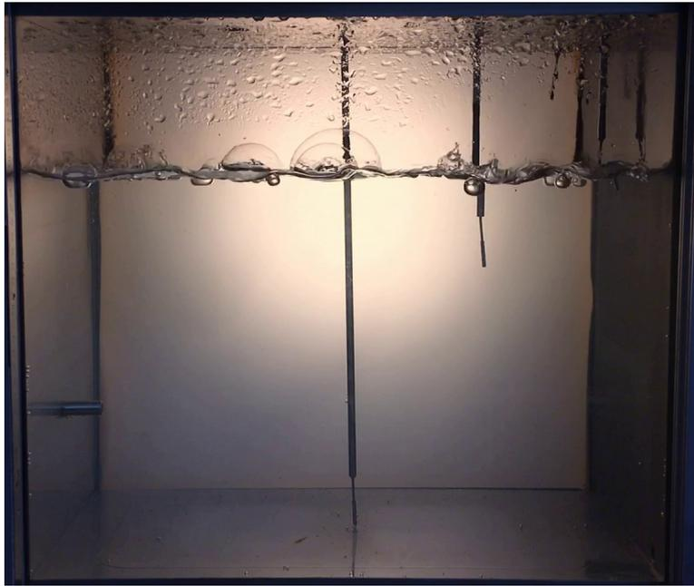
Figure 3.13: During the first stage of the test and when the initial strong bubbling originating from the heated wall ceased, water continuously turned into bubbles just below the liquid free surface.
