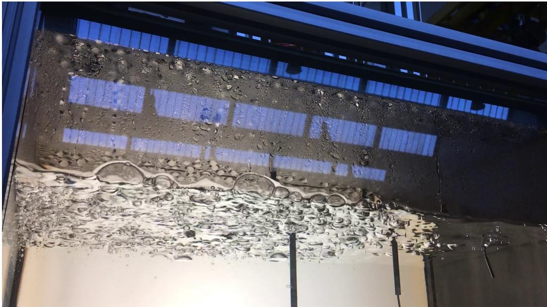
Figure 3.29: A photo taken during Stage 3 of the step-by-step test performed in December 14, 2021. The image shows the same kind of fast and sometimes explosive bubble growth as during the reference test.
