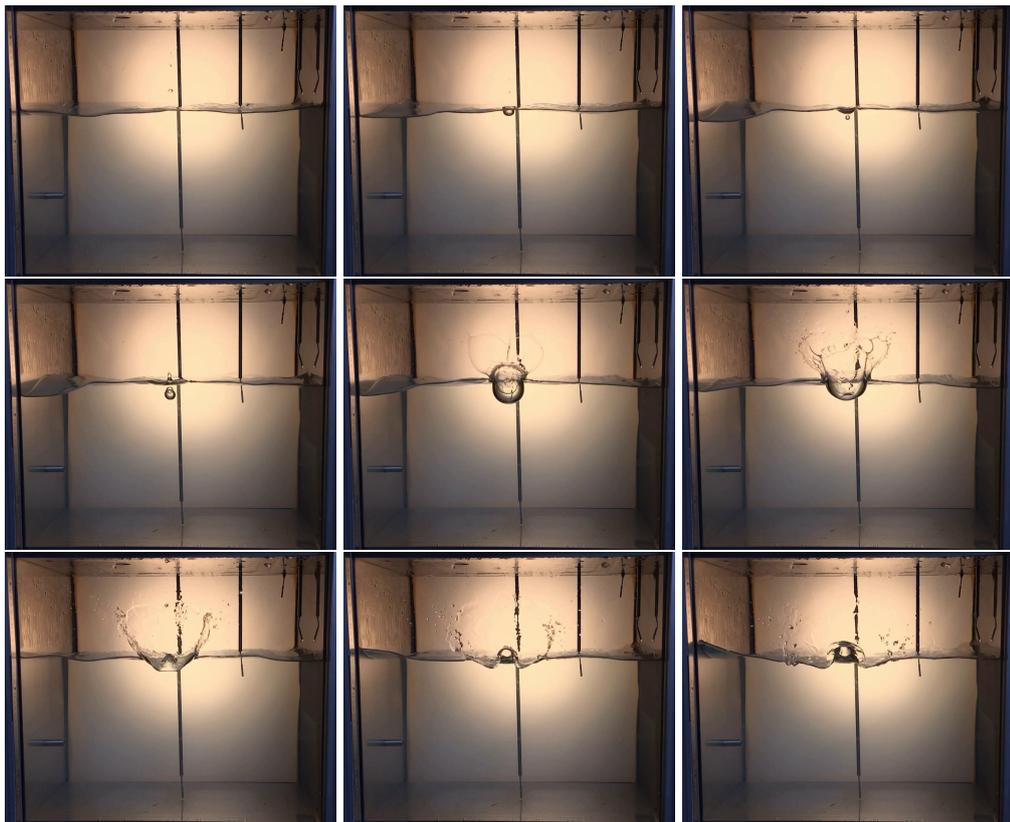
Figure 3.15: A series of photos taken during the late stage of the reference test. The pictures are displayed every 4 ms. The series shows the interaction of a falling droplet with the liquid free surface. The interaction leads to the violent nucleation of a bubble.
