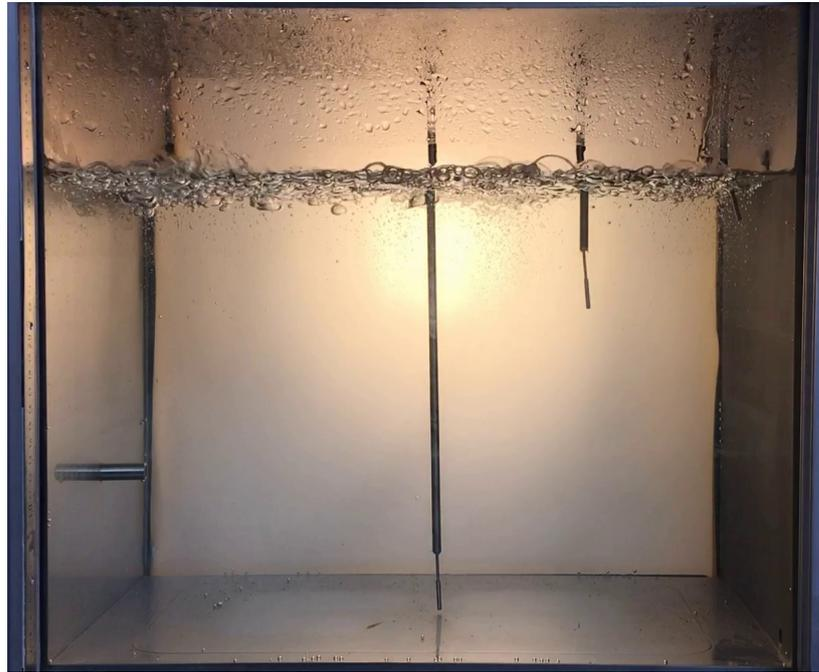
Figure 3.41: A photo taken during the first minute of the test conducted at a power of 1000 W and a pressure of 42 mbar, exhibiting some strong bubble flashing underneath the liquid free surface. One can notice that at the time of the photo, the bubble nucleation has ceased onto the heated bottom wall of the vessel.
