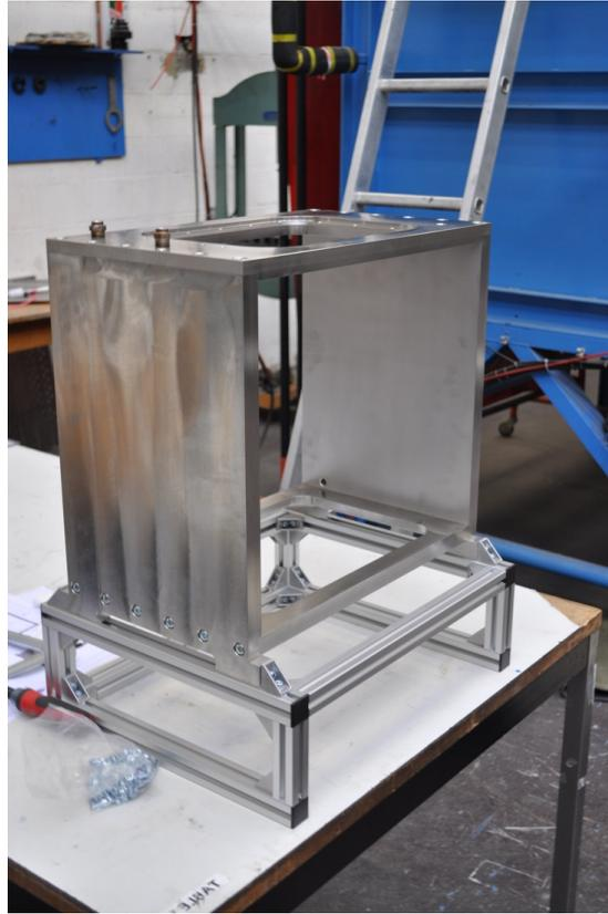
Figure 2.8: Side-view of the mechanical assembly of four machined stainless steel plates constituting the Aquarius pool vessel.
