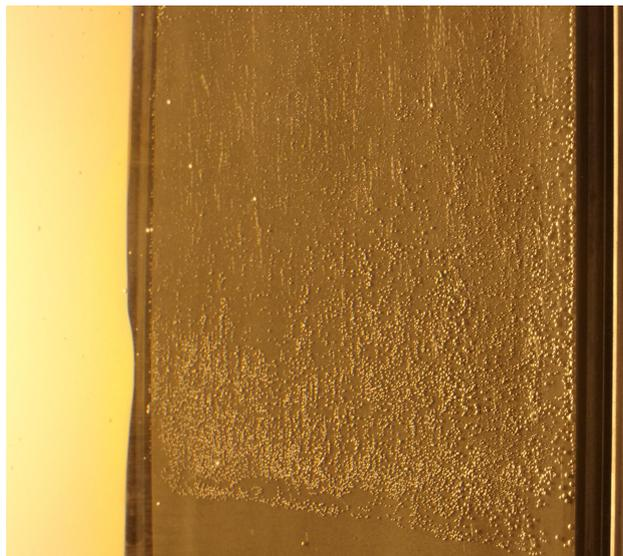
Figure 3.61: A study of the forcing of bubble nucleation onto the unheated rough wall of the vessel. Photo taken right after the beginning of the test conducted at a power of 250 W, a pressure of 22 mbar, an initial dissolved  $O_2$  concentration of 9.5 mg/L, an initial pool level of 30 cm and a prior dry out of the unheated rough wall. Numerous bubbles are visible, thereby validating the retained forcing experimental procedure.
