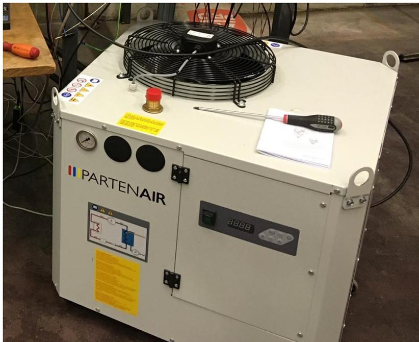
Figure 2.13: Front-view of the Partenaire™ FRC-VBE 003 air/water heat pump equipping the test device.
