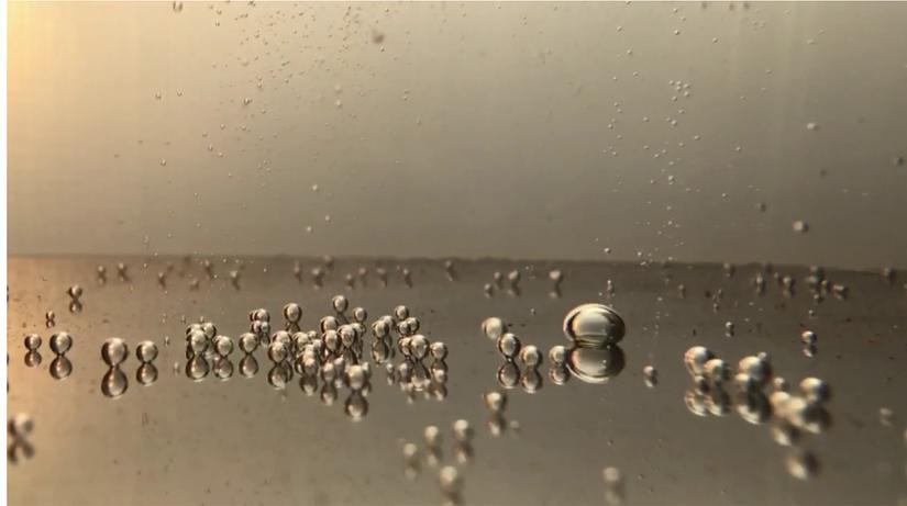
Figure 3.8: A close look at one mushroom-like shaped centimetric bubble, nucleated onto the heated wall (here located close to the center of the image), at the beginning of the reference test.
