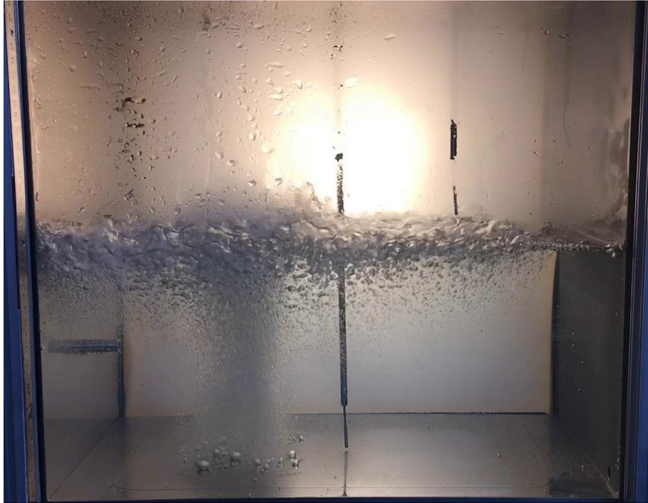
Figure 3.48: A photo taken 10 s after the beginning of the test conducted at a power of 1000 W, a pressure of 22 mbar, an initial dissolved  $O_2$  concentration of 6.5 mg/L and an initial pool level of 20 cm, exhibiting some strong flashing underneath the liquid free surface and a not less intensive bubble nucleation onto the vessel's heated bottom wall.
