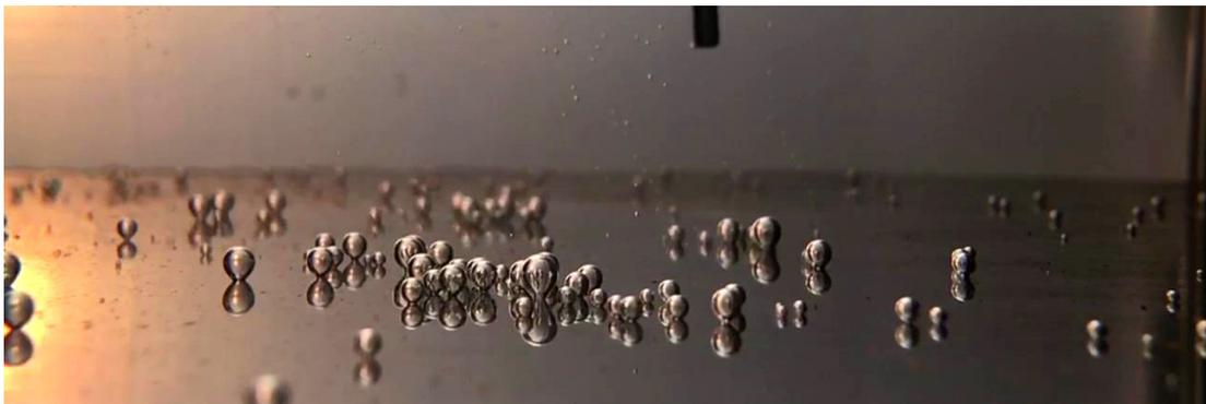
Figure 3.3: A close look at the heated wall of the pool vessel, showing numerous processes of bubble nucleation.
