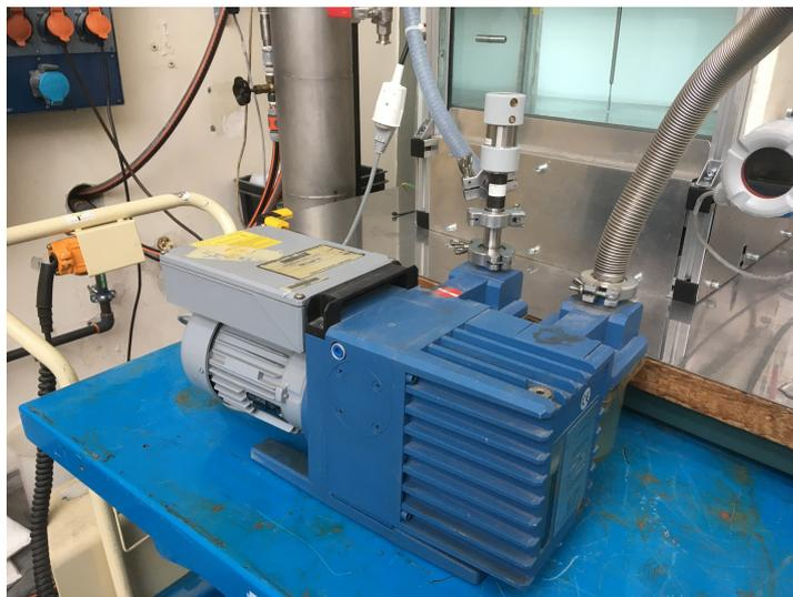
Figure 2.9: Side-view of the Vacuubrand™ RE 8 vacuum pump in use within the Aquarius test device.
