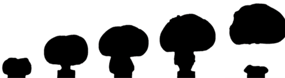
Figure II.5- Experimental observation of bubble formation process
