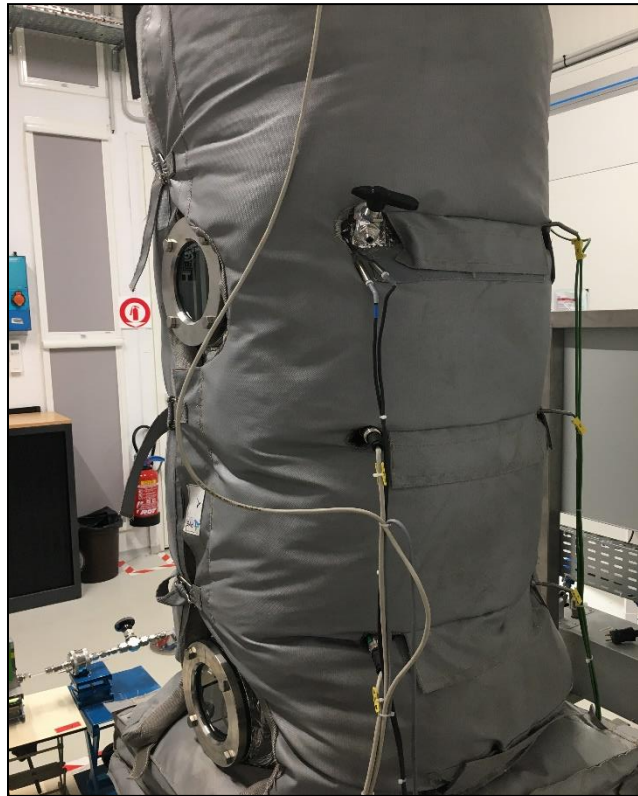
Figure II.8- Pressure and temperature sensors plugged to TYFON column.
