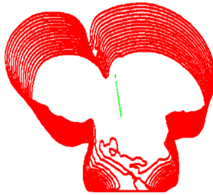
Figure III.32- Tracking the center of gravity of globule during its formation and rising.
