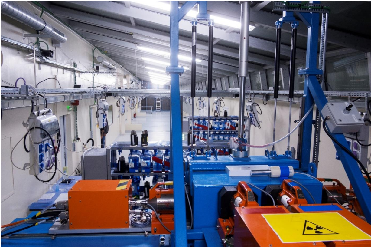
Figure 19 – Irradiation Hall – MICADO'Lab with 4 sources (orange boxes) and fish racks.
