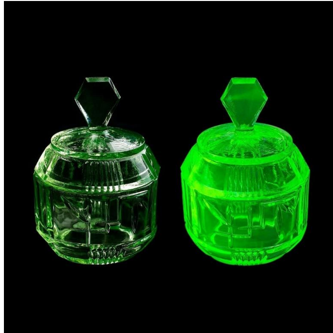
Figure 3 – Uranium glass under visible light (left) and under ultraviolet illumination (right). From “Uranium glass fluorescing – 11725688 | Science Photo Library,” n.d.
