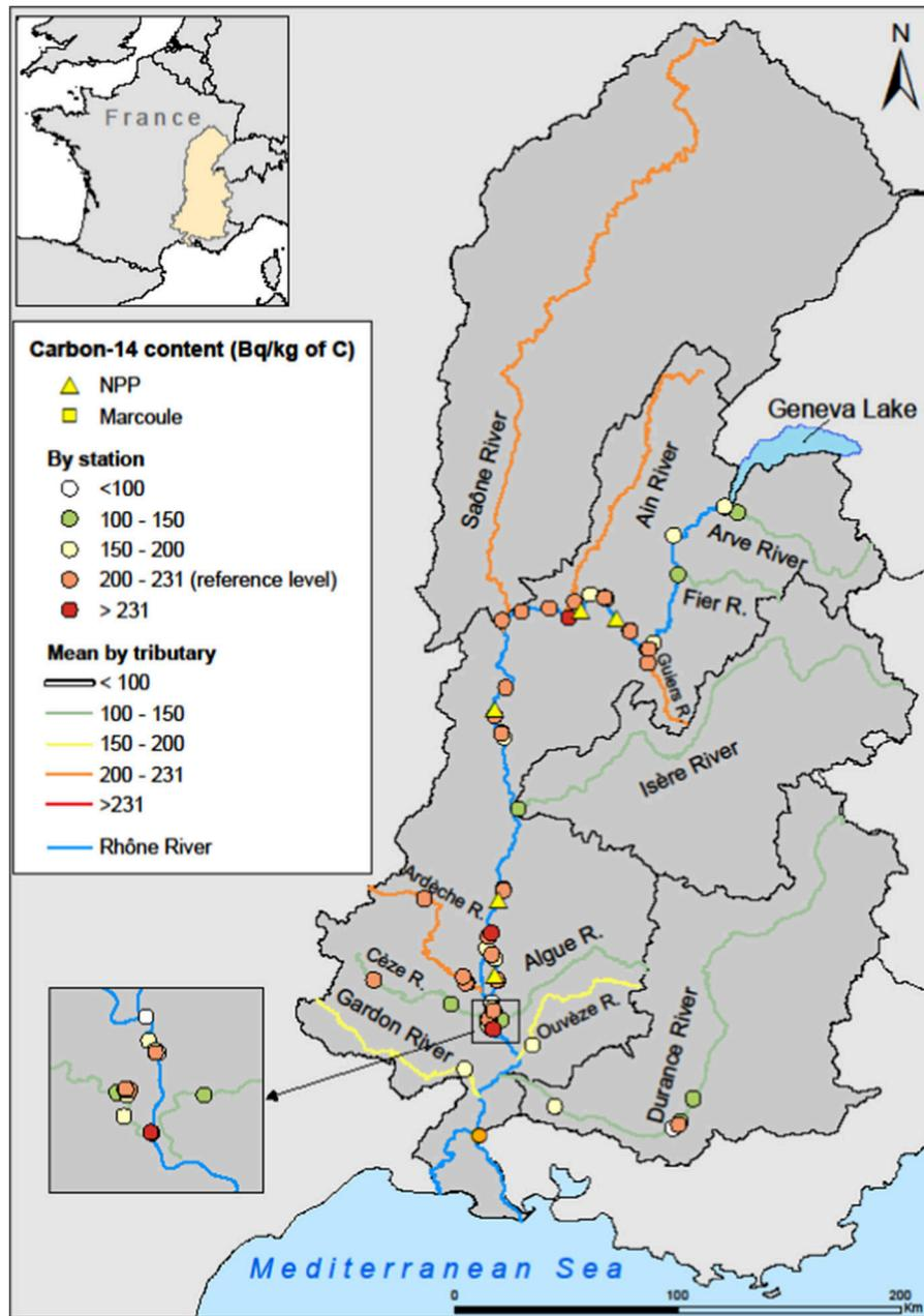
**Fig. 8.**  $^{14}\text{C}$  contents (Bq/kgC) in sediments of the Rhône watershed over the last 10 years (2007–2017). Data acquired most usually near tributary confluences with the Rhône River are generalized to the whole tributary watershed.
