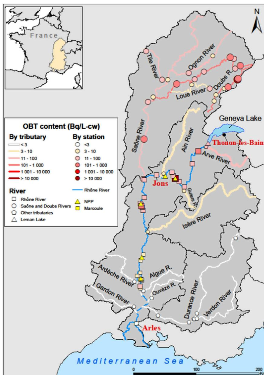
**Fig. 5.** OBt levels (Bq/L) in sediments of the Rhône watershed over the last 10 years (2007–2017). Data acquired most usually near tributary confluences with the Rhône River are generalized to the whole tributary watershed.
